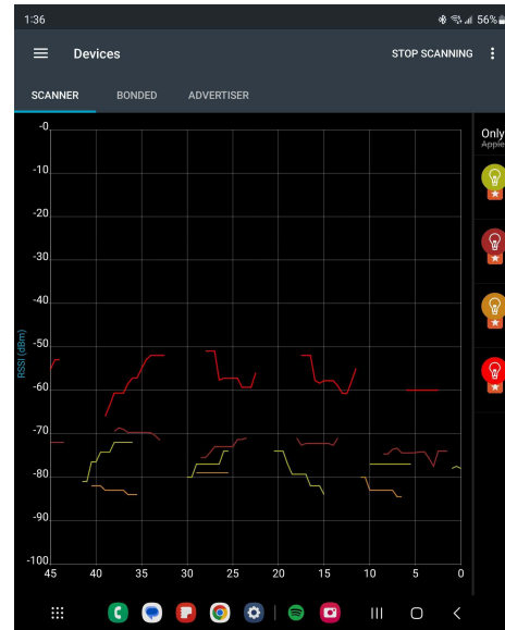
FIGURE 24. In-medium bench comparison of MIT- and TRT-built devices. Left: the physical arrangement. Four devices hang in a water-filled beaker on a common support. A bench nRF development board logs RSSI and temperature per device over serial. The smartphone that took the photograph also ran the concurrent scan, and its case sits empty on the bench. Right: the smartphone nRF Connect scan of the same four devices from that position. The comparison sets one MIT-built device (A902) against three TRT-built devices (B106, B107, B128) under identical immersion and scan geometry. The two builds differed only in the 3D-printed spacer surrounding the antenna and were otherwise identical. It therefore reads as a qualitative build-to-build comparison rather than a calibrated link measurement. The smartphone reports uncalibrated RSSI, and orientation moved by hand between readings.
