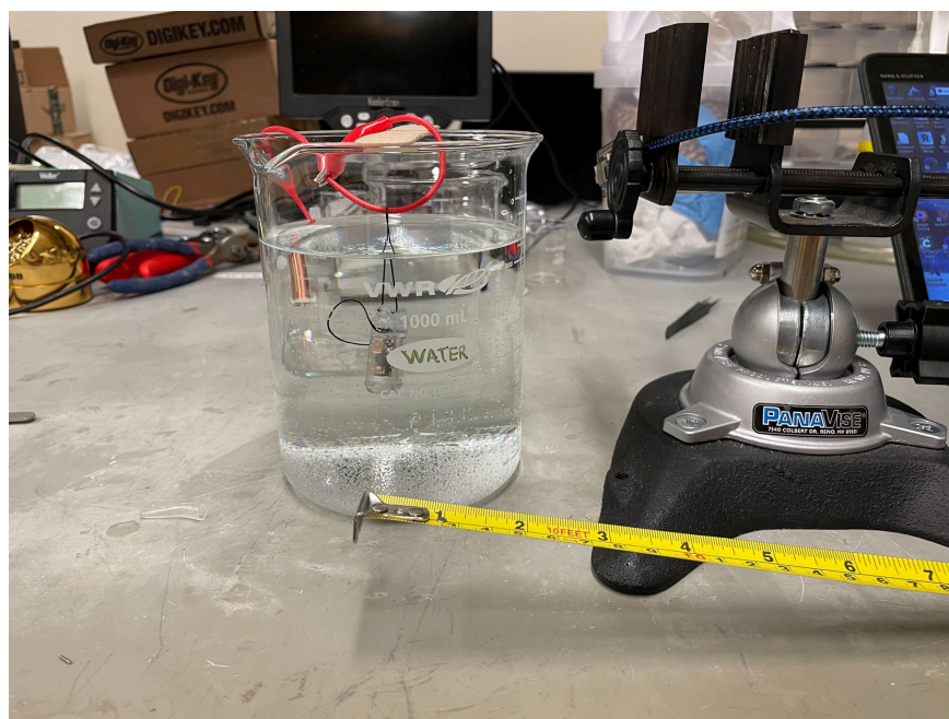
FIGURE 8. Water-phantom bench setup. A capsule hangs on a thread at mid-depth in a 1000 mL beaker of water, the surrogate medium for these runs. A tape measure sets the separation to the receiver held in the bench vise, which makes the geometry repeatable between runs. Water loads the antenna somewhat harder than muscle at 2.4 GHz, so this arrangement is a repeatable bench check rather than a tissue-equivalent reproduction of in-body loading. Routine large-animal access meant in-body behavior could be confirmed directly, so a formulated phantom was not required.
